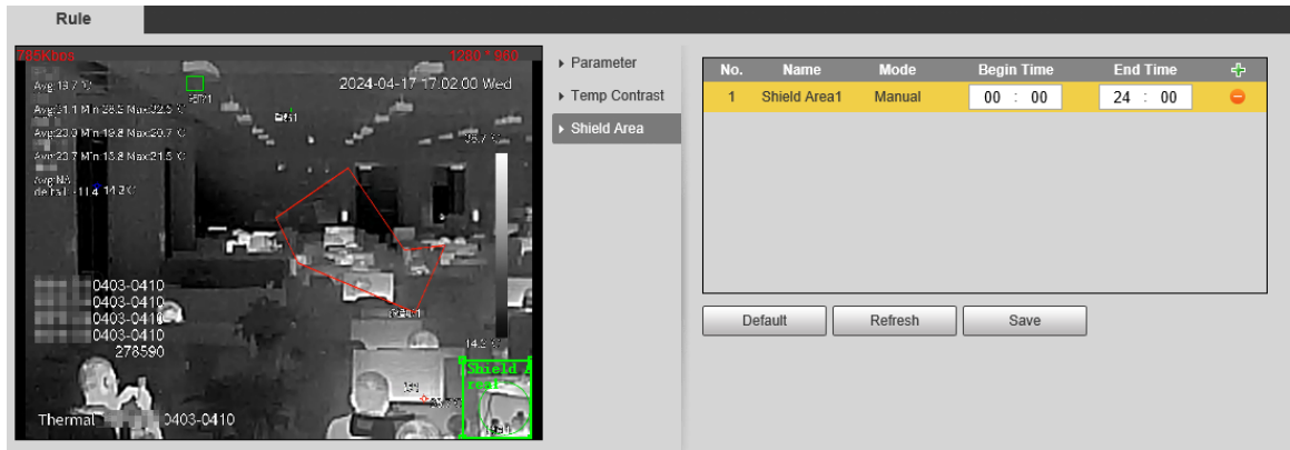
Figure 5-27 Configure shield area
